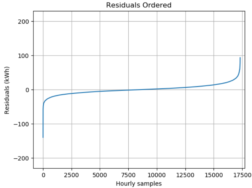
Figure 9: The residuals of LR and FFNN when estimating the load of all stations part of the test set. The data estimated comes from stations that have been used for training LR and FFNN. However, the hours which are estimated have not been seen by LR and FFNN in training
